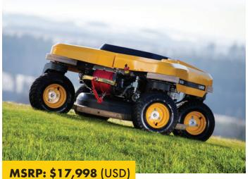
The SPIDER CROSS LINER is sure to impress with its innovative and compact design. This well-equipped commercial lawn mower features a terrain-copying platform, integrated stabilizing winch, and skid-steering option.
